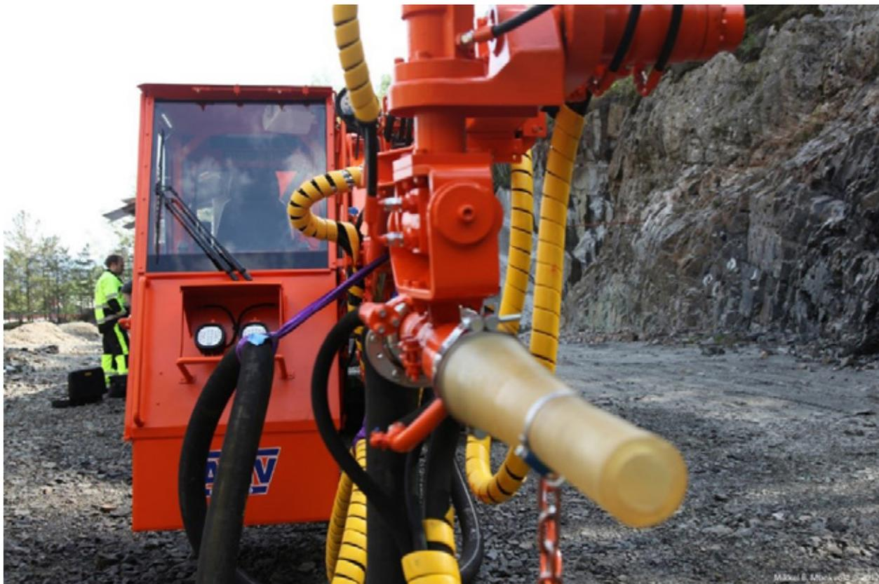
Figure 1.3.16: Shotcrete operator cabin with extended arm and nozzle [11].
