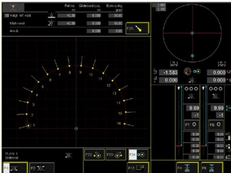
Figure 1.3.31: Interface of the tracking system for technical bolts. The blue dot in the crosshair in the upper right corner shows the position of the drill bit versus the placement of the drill hole (Bever Drill).
