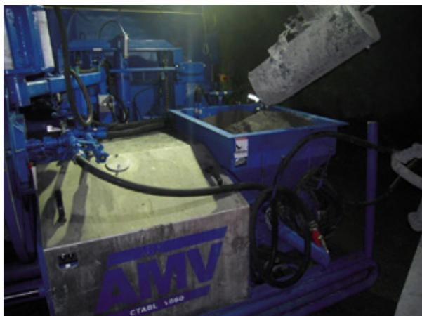
Figure 1.3.17: Shotcrete rig with shotcrete pump and concrete receiving hopper.
