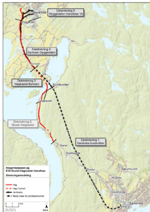
Figure 3.1.1: An overview of The Ringerike Line and E16 Highway (FRE16). Dashed black line shows where the railway tunnel is planned, between Sandvika and Sundvollen (23 km), and between Sundvollen and Bymoen (3 km).
