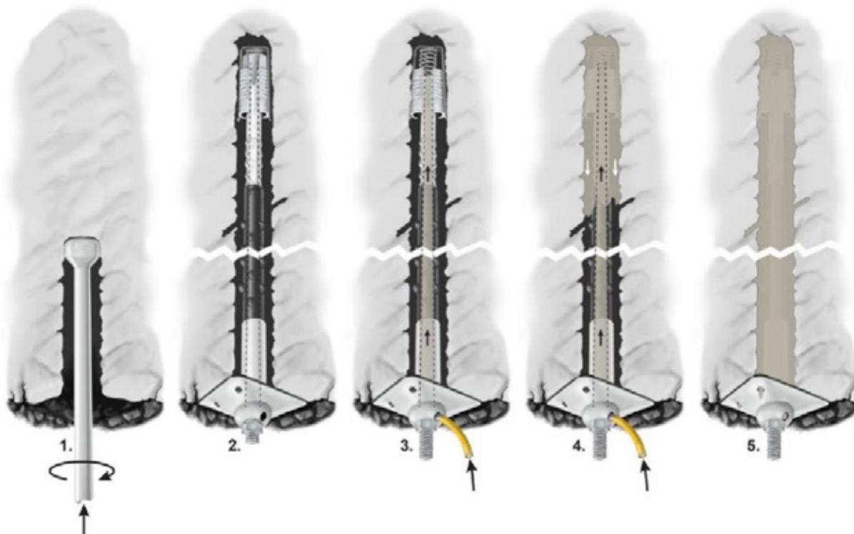
Figure 1.3.22: 1. The hole is drilled as long as the length of the bolt. 2. The bolt is installed with an expansion shell and are point anchored to ca. 50 kN. It is considered a temporarily anchored bolt until it can be fully grouted. 3 and 4. The casting is done by plugging a tube in to the sphere in the bolt and it can now begin to pump in cement. 5. Fully grouted bolt [14].
