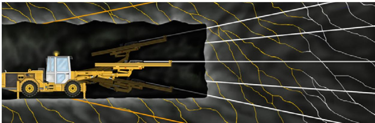
Figure 1.3.7: Pre-grouting. Holes are normally drilled with a length of approximately 24 metres from the tunnel face [7].
