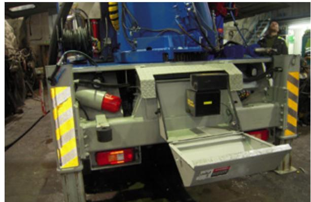
Figure 1.3.20: Profiler mounted on the shotcrete rig for scanning of the tunnel walls for accurate thickness measurement of shotcrete.
