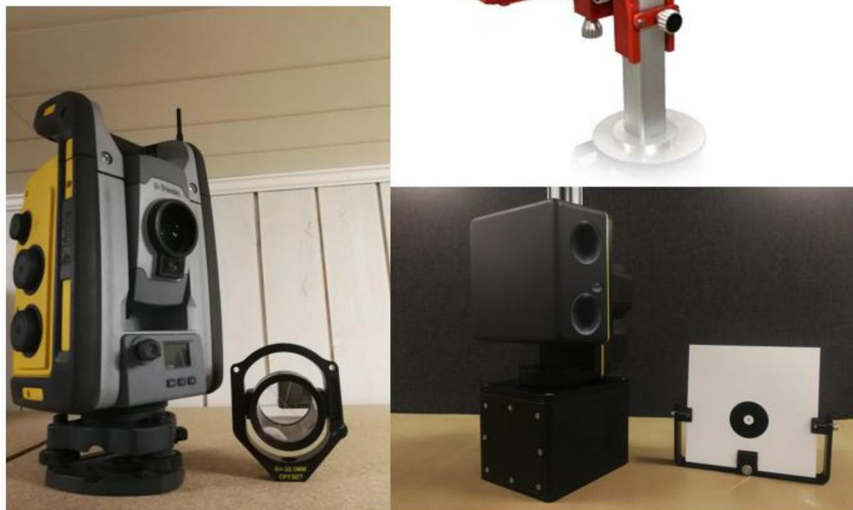
Figure 1.3.4: Upper right image shows a tunnel laser [2], lower left image shows a total station with a prism, lower right image shows a profiler with a target plate.
