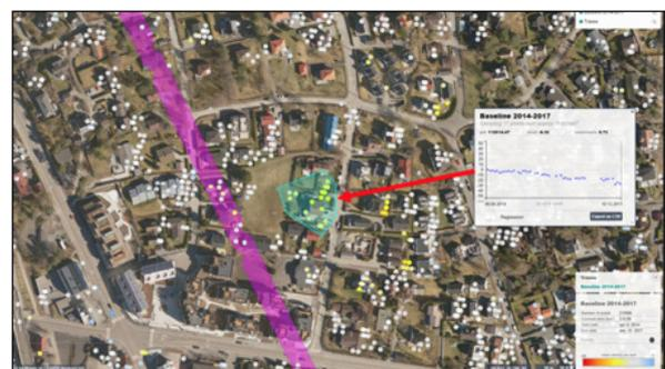
Figure 1.6.6 shows a zoom-in of one region along Follo Line. The blue structure examples an area where settlements can be observed. The time series show that the settlements started before the onset of the Follo Line construction. It also indicates a recent acceleration of the settlement velocity.
