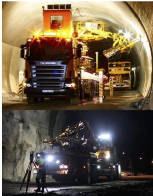
Figure 1.3.30: AMV Bolt rigs for technical installations.
