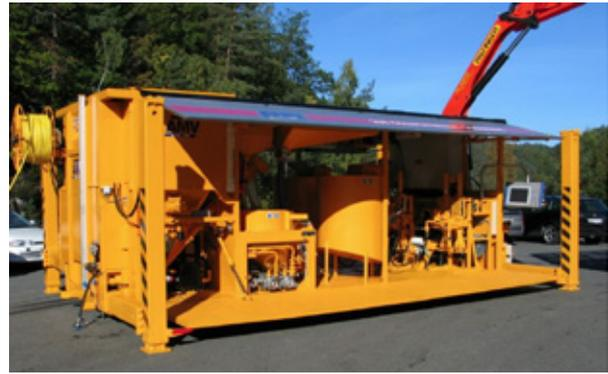
Figure 1.3.11: AMV Grouting rig is equipped with silos, mixers, agitator and pumps. These are standard for modern grouting rigs.
